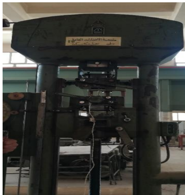
Fig.4. an electronic universal testing machine
